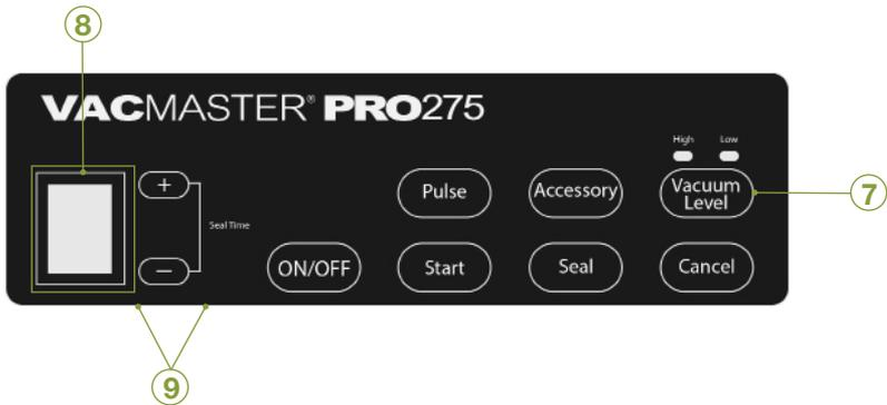
**7 Vacuum Level Button** - Press the “Vacuum Level” button to set the vacuum level needed. There are two options - High or Low. The default setting is high.
